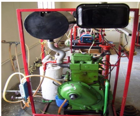
Fig.1.diesel engine test ring
